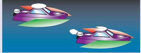
Note: if vessel is less than 12 m long, sidelights may be a combined lantern on the fore and aft centreline.
