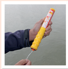
Step 2: Hold vertically above head, pull sharply on ball to fire.
